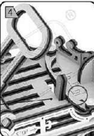
**EN** Insert the key and start the rubber motor rotating of the key on 20 rotations in a clockwise manner;
